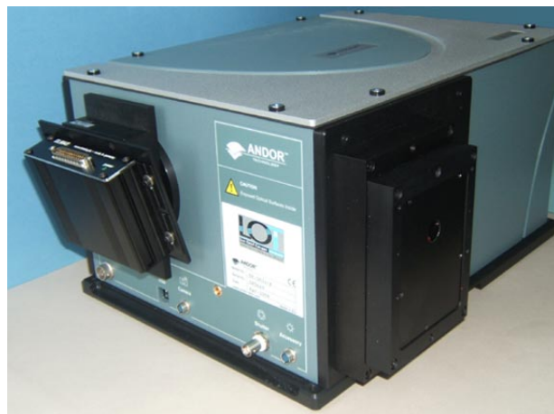
Shamrock SR303 Spectrometer with DL9840
